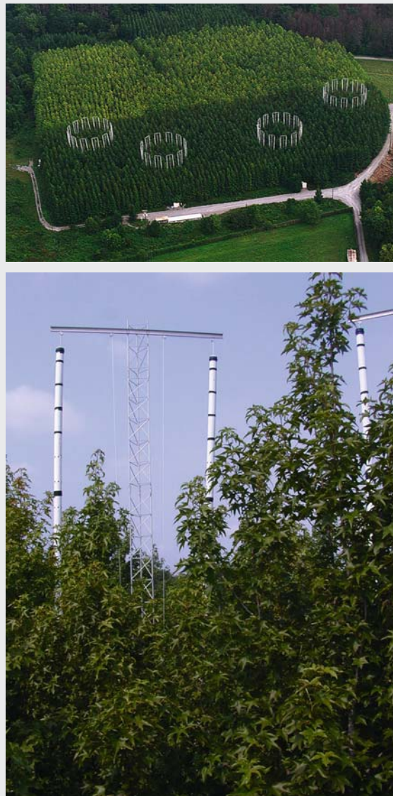
Fig. 4.14. The FACE (Free-Air Carbon dioxide Enrichment) experiment in a stand of Liquidambar styraciflua (sweetgum) trees at Oak Ridge National Laboratory, USA
