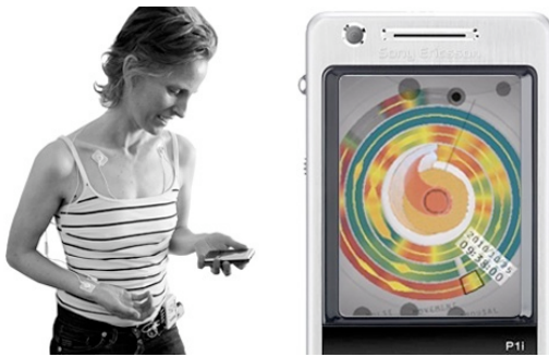
Figure 1. The sensor placed on the body and the visualization of the Affective Health mobile application
